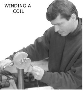
From now on you need to keep hold of the wire(s) with one hand and the handle of the winder with the other hand. Keep a gentle tension in the wire(s). If you release the wire then the coil may lose its shape and be impossible to salvage.
