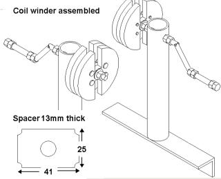
You will also need to make a spacer that keeps the two cheek pieces the correct distance apart. This should be 25 x 41 mm with corners cut off to fit between the pins. 13 mm thick (or 10 mm thick for the 1200 turbine). You can adjust the thickness if the first coil attempt does not fit the stator. Drill a 10 mm diameter hole at the exact centre.
